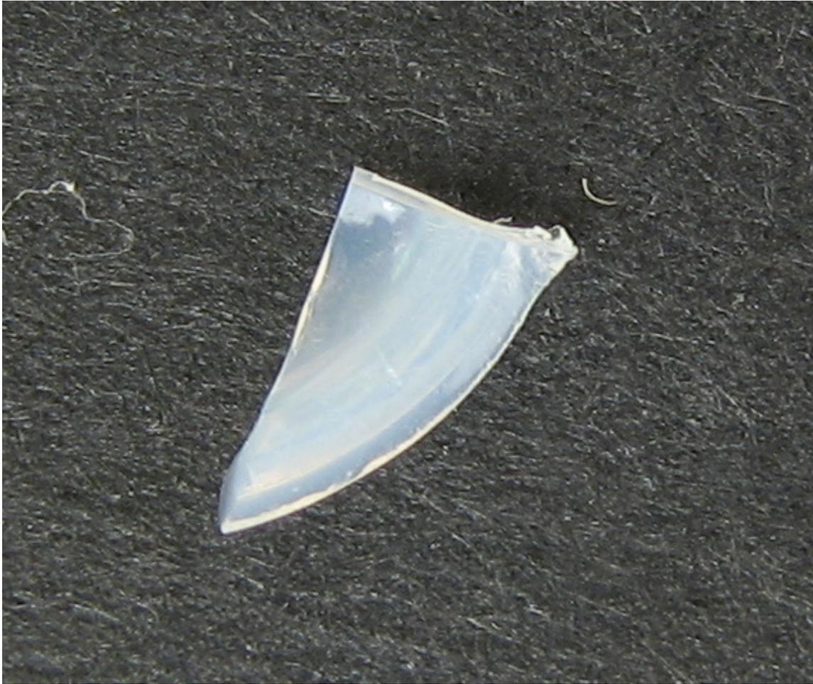
Figure 2.2: A small, sample monolith of alumina. Note the blue sheen, which is characteristic of Yoldas alumina sol-gels.
