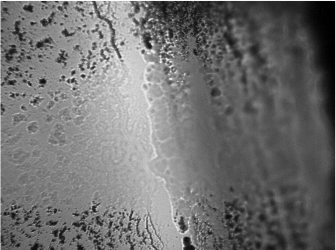
Figure 3.5: An edge-on, 400 $\times$ , transmission-lit view of the film in Figure 3.4. The film is so thin, its breadth cannot be seen at this magnification. At the edge of the laser-densified region, some melting of the glass substrate can be seen.
