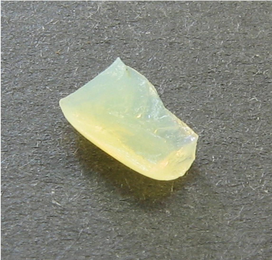
Figure 2.3: A typical, fully-cured sample of alumina made through the Yoldas sol-gel process. The yellow tint is a sign of the chromium doping.
